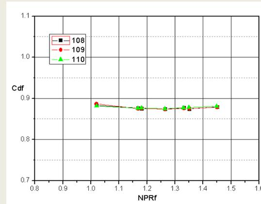
(b) the discharge coefficient of the fan
