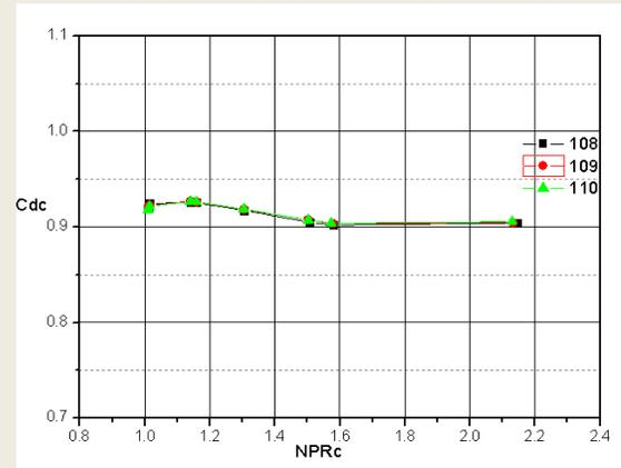
(a) the discharge coefficient of the core
