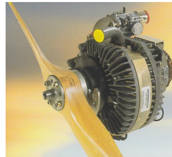
28.3kW AR 741 rotary engine
